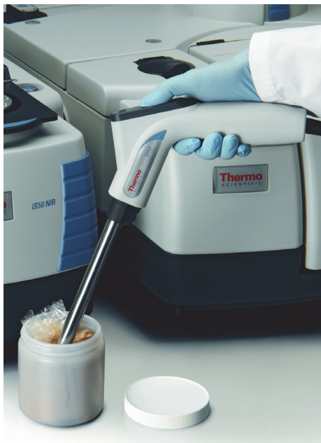
Figure 15. Sample ready for measurement with the SabIR probe
