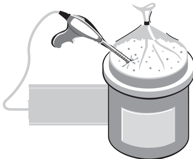
Figure 16. Powder sample ready for measurement with a diffuse reflection probe
