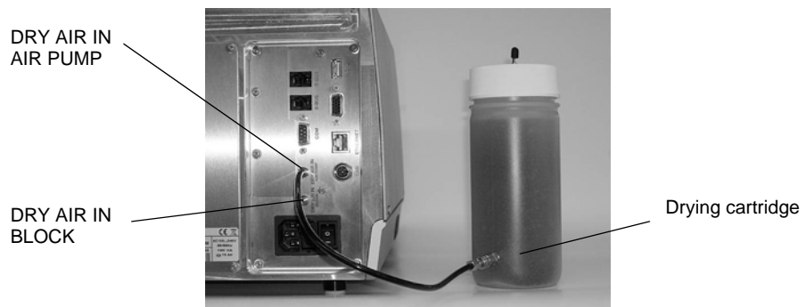
Fig. C - 1 Drying cartridge connected
