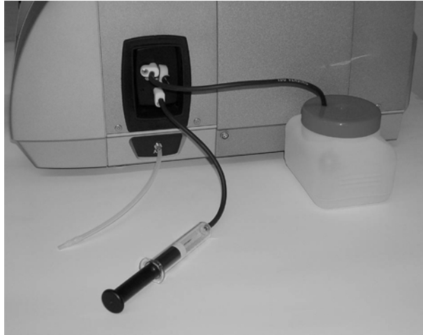
Fig. 13 - 2 Filling with a glass syringe
