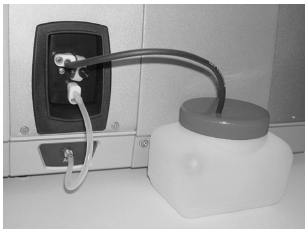
Fig. 7 - 3 Placing the waste vessel
