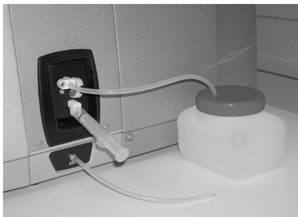
Fig. 13 - 3 Filling with a plastic syringe
